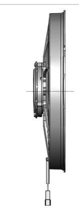
High Power fans have a deeper profile motor requiring more clearance and draw a higher current, these are suited to applications demanding a higher airflow or high density/thicker cores (50mm+) or vehicles fitted with air conditioning condensers in front of the radiator.
