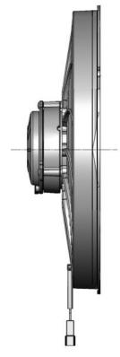
Very High Power fans have an even deeper profile and draw a higher current and have an even higher airflow, especially through higher density/thicker cores (75mm+) or intercooler, condenser and radiator packages.
